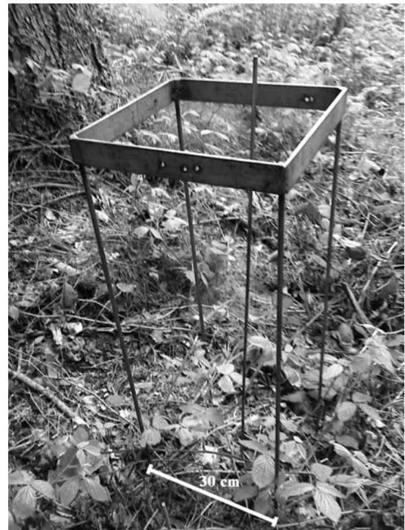
Figure 1 Four welded rods and two free rods (only one is shown on the photograph) were used to estimate the LAI of bramble thickets. The whole system was pushed vertically into the thicket and the number of hits between the rods and canes or leaves were counted and related to bramble LAI (Figure 2).
