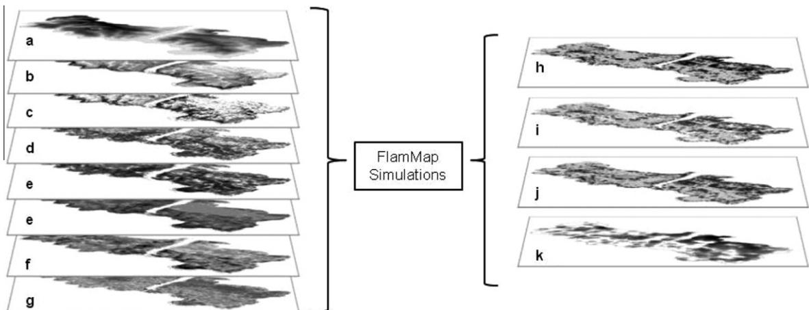
Fig. 2. Input layers required to run FlamMap: (a) elevation, (b) slope, (c) aspect, (d) fuel model, (e) canopy cover, (f) canopy base height, (g) canopy bulk density and selected output layers obtained from FlamMap, (h) crown fire activity, (i) flame length, (j) heat/fireline intensity, (k) burn probabilities.
